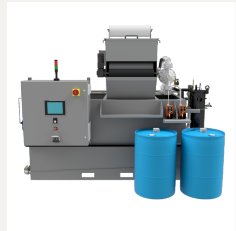
FRONT - CHEMICAL DOSING AND HMI
